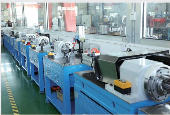
电主轴检测线 Electric Spindle Test Machines
