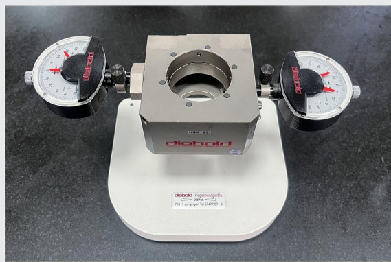
1: 10锥度检测工具图 (德国戴博刀柄检具) Picture of 1:10 taper inspection tool (German Daibo collet chuck inspection tool)
